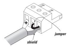
Terminal block: unbalanced connections
